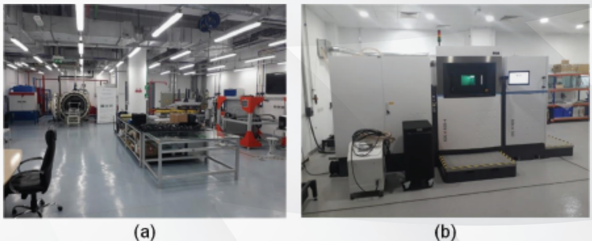
Figure 1: (a) Photograph of the ARIC laboratory and (b) the EOS 400-4 additive manufacturing machine.
